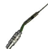
Thermocouple type K for wall measurement
